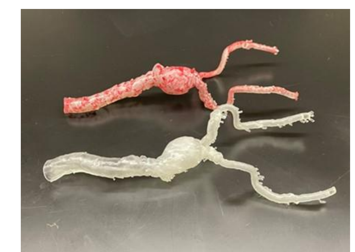
Figure 1: 3D Print of an Abdominal Aortic Aneurysm. Printed on a FormLabs 3 printer in flexible material.
