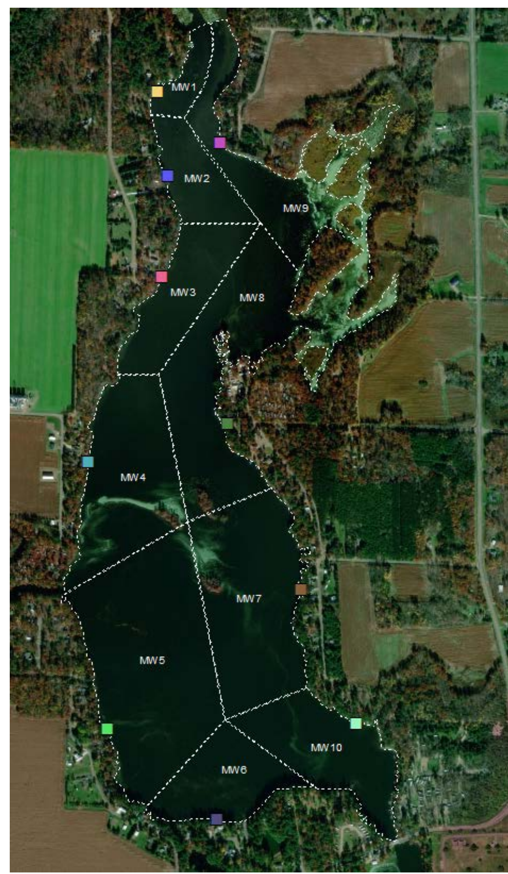
Figure 4. Map showing mini-piezometer locations and representative lake segments for each piezometer.
