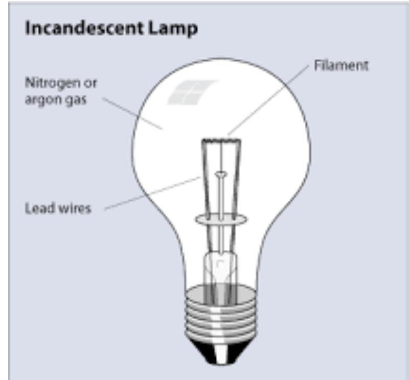
The incandescent lamp is the oldest and most common type of lamp. Light is emitted when electricity flows through—and heats—a tungsten filament.
